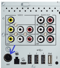
Parrot ASTEROID Smart antenna Example of antenna adaptor -DIN / Fakra (not provided) connector
